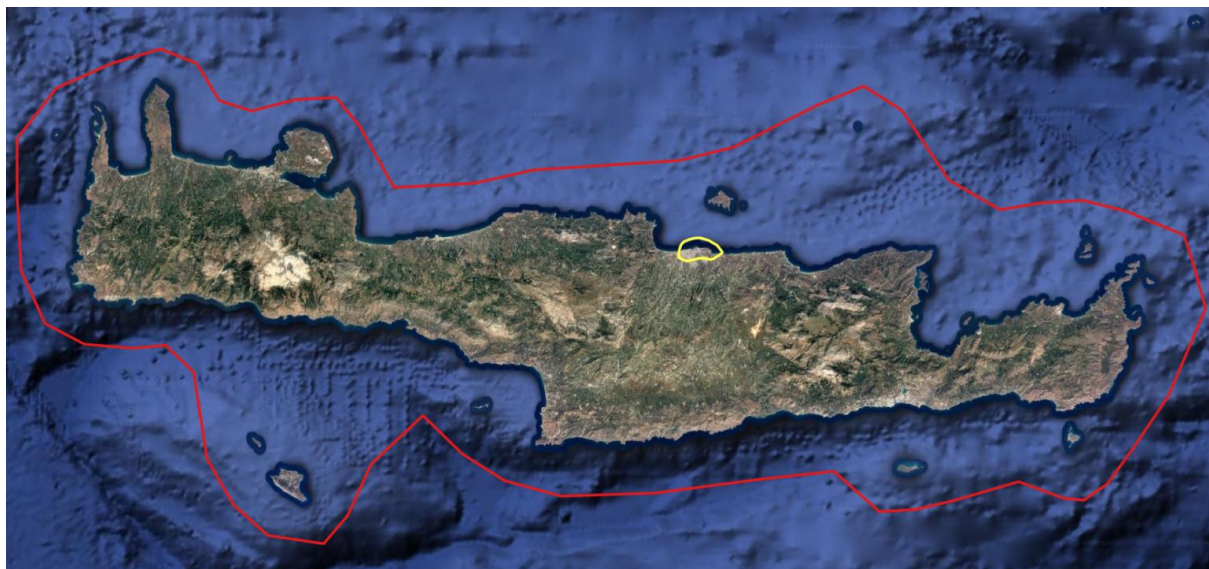
Figure 15. Polygon geometries of selected areas of interest. (a) Red boundary is used for clipping the whole Crete Island; (b) Yellow boundary is used for clipping the coastal area around the Port of Heraklion.
